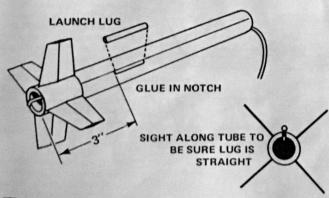
**7** Glue the launch lug (part J) to the body tube between two fins, 3" ahead of the rear of the model as shown. (Use white glue.) Sight along the tube to be sure the launch lug is straight on the body.
