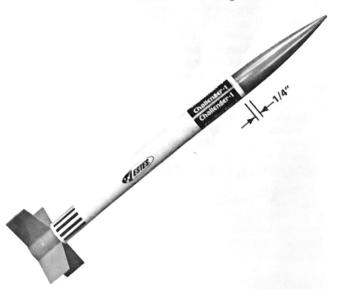
■ 10 Apply decals (part G). Cut out a decal section, dip it in lukewarm water for 10 seconds, and hold it until it uncurls. Slip the decal off the backing sheet and onto the model. Blot excess water away. Apply all decals as shown in the photograph. For best results, let the model dry overnight and apply a coat of clear spray to protect the decals.
