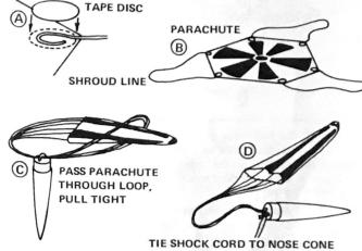
**9** Cut out the parachute (part L) on its edge lines. Cut three 24 inch lengths of shroud line (part M). Attach line ends to the top of the parachute with tape discs (part N) as shown. Pass the shroud line loops through the ring at the rear of the nose cone. Pass the parachute through the loop ends and draw lines tight against the ring. Set the knot with a drop of glue. Tie the free end of the shock cord to the ring.
