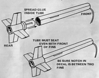
Spread white glue around the inside of the body tube at the end opposite the shock cord mount. The glue should cover an area extending 1/2 inch into the tube. Insert the front of the fin unit into the rear of the body tube. The tube should "seat" evenly and tightly against the shoulder on the fin unit.
