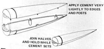
Glue the two nose cone halves (part K) together using plastic model cement. Be careful to not use too much or you will have a sloppy-looking joint. Make sure the alignment pins on the inside of the cone fit completely into their matching holes.
